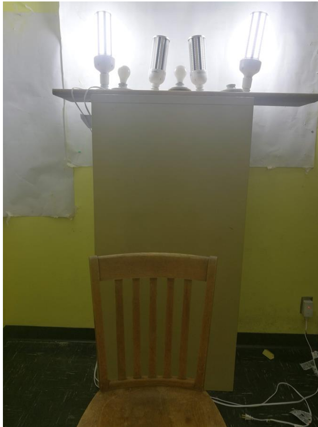
Figure 3 : Cool light (Blue at 450 nm ) set up on wooden plank and with a subject chair facing away from the light
