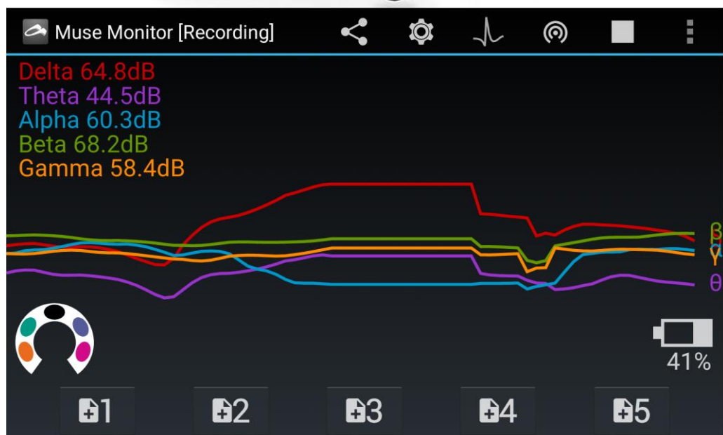
Figure 1: (a) Muse Headband. (b) Muse recording streaming through Muse Monitor app. Top left corner shows brain waves of delta, theta, alpha, beta, and gamma. Lower left corner with the horseshoe represents signal strength at 5 electrodes.
